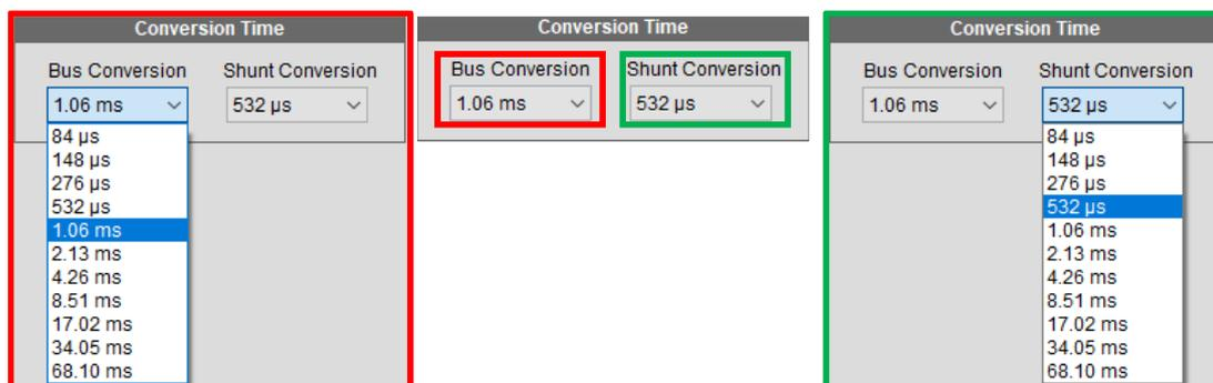
Figure 22. Bus/Shunt Conversion Time Settings
