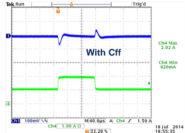
1. Apply a fast step load and if it shows ringing, measure the ringing frequency
