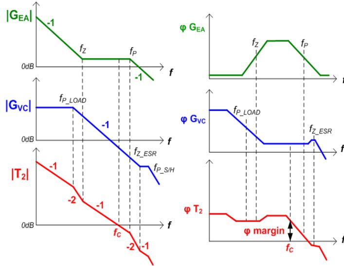
$$f_{P\_LOAD} = \frac{1}{2\pi C_{OUT} \cdot R_{LOAD}}$$
