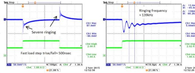
**Quickly check converter loop stability**
