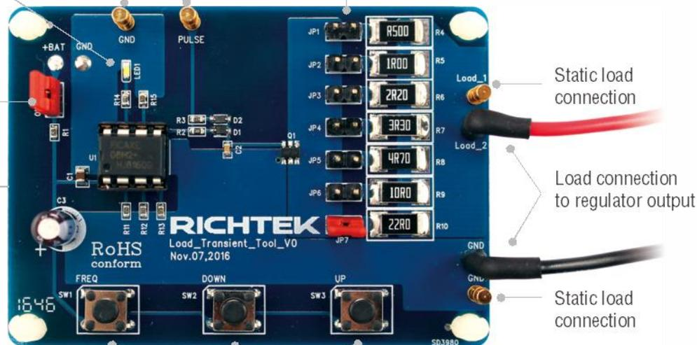
Press UP or DOWN button: Duty-cycle adjust 0.1% ~ 50%
