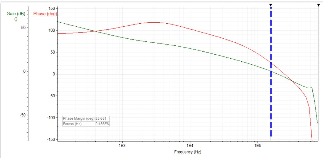
Circuit simulation using online Richtek Designer tool and using 16 $\mu$ F output capacitance confirms the step load result:
