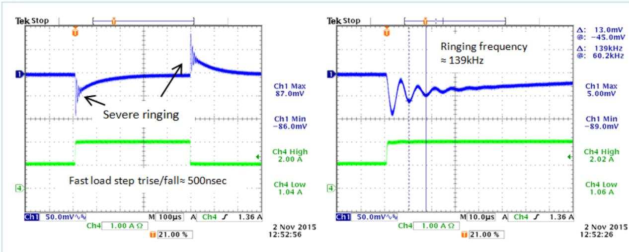
Step load shows severe ringing with ringing frequency of 139kHz
