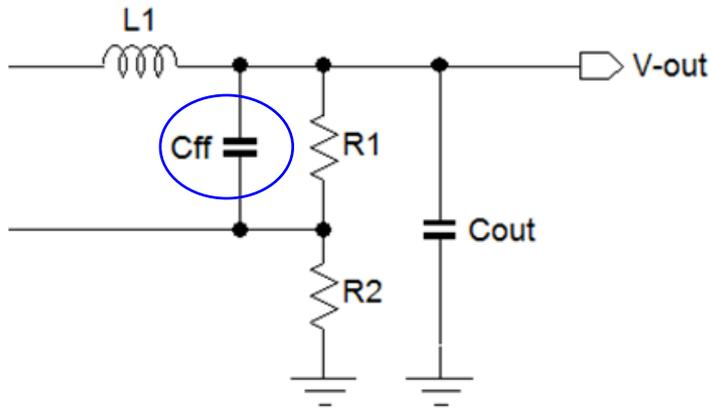
The feed-forward capacitor plays a role in the damping of the ACOT control loop, especially at higher duty-cycle applications like 12V → 5V. For low duty-cycle applications like 12V → 1V it is normally not needed. The value of Cff for a specific ACOT converter depends on duty-cycle, C<sub>OUT</sub> value, inductor value and R1 value.
