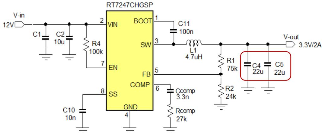
800kHz converter designed for 2x22uF output capacitance in 3.3V output application.
