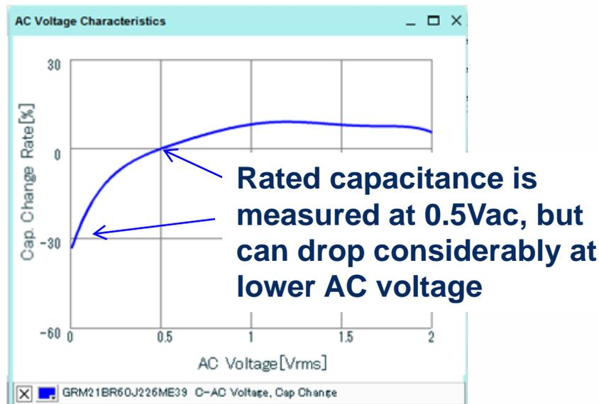
(if DC bias or AC voltage effect is not specified for your capacitor type, ask for it)
