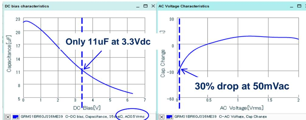
Actual capacitance is  $11\mu\text{F} * 0.7 = 8\mu\text{F}$ : total output capacitance **16uF instead of 44uF**
