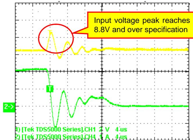
Figure 2. RT9711 power switch operated in worse condition:
