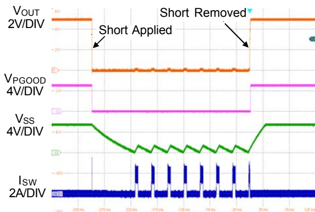
Figure 3. Short-Circuit Protection and Recovery
