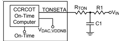
Figure 18. VDDNB Controller : On-Time Setting with  $R_C$  filter
