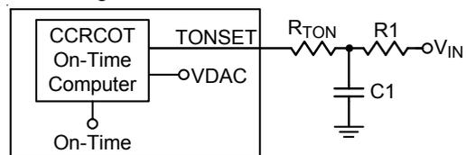
Figure 11. VDD Controller : On-Time Setting with R<sub>C</sub> filter
