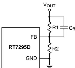
Figure 1. C<sub>ff</sub> Capacitor Setting
