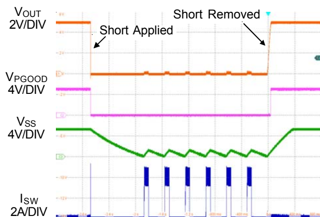
Figure 3. Short-Circuit Protection and Recovery
