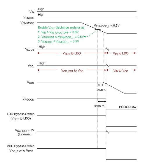
Figure 8. The RT6320B/BH EN/MODE Pin Power Off
