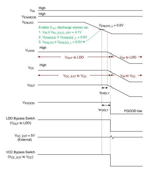
Figure 11. The RT6320C/CH ENLDO Pin Power Off
