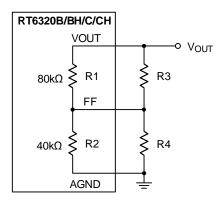
Figure 12. RT6320B/BH/C/CH Slightly Adjusts Vout with FF Pin
