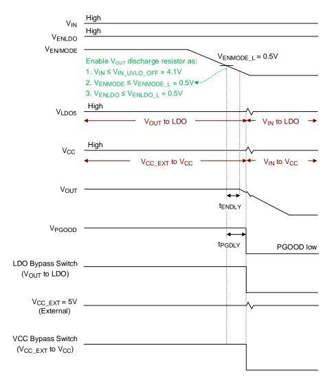
Figure 9. The RT6320C/CH EN/MODE Pin Power Off
