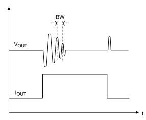
Figure 16. A Simple Way to Get the Bandwidth Following the above concept, the equation of bandwidth with feedforward CFF is derived, as expressed in equation (5).
