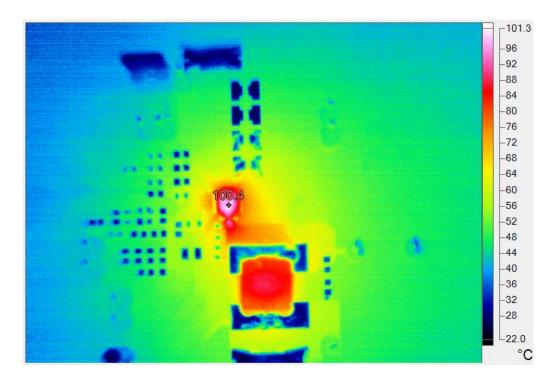
Figure 20. Thermal image of RT6320B/BH with Vout = 3.3V, VIN = 19V, IOUT = 12A and VCC EXT = 5V
