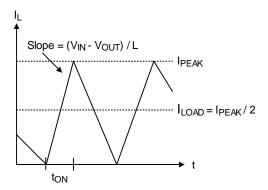
Figure 2. Boundary Condition of CCM/DEM
