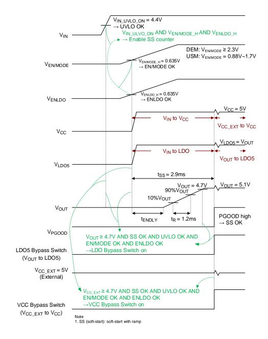
Figure 5. The RT6320C/CH VIN and EN/MODE Pin Power On
