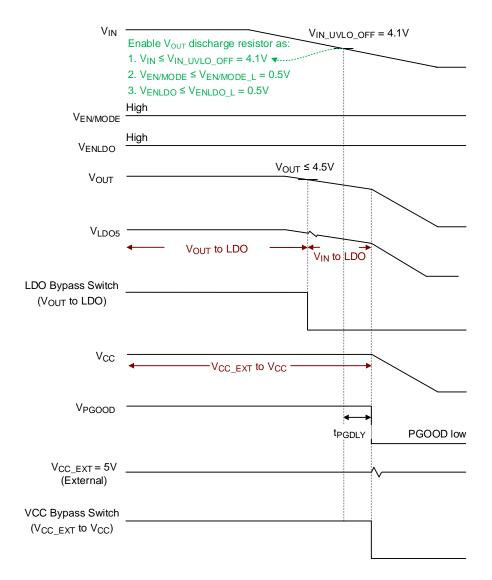
Figure 7. The RT6320C/CH VIN Pin Power Off
