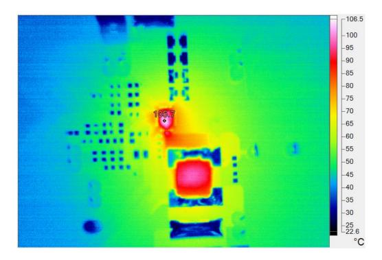
Figure 21. Thermal image of RT6320C/CH with Vout = 5.1V, VIN = 19V, IOUT = 12A and VCC EXT = 5V
