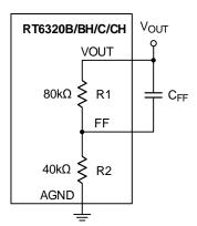
Figure 14. RT6320B/BH/C/CH Feedback Loop with Feedforward Capacitor
