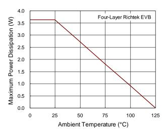
Figure 17. De-rating Curve of Maximum Power Dissipation
