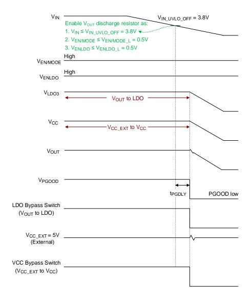
Figure 6. The RT6320B/BH VIN Pin Power Off
