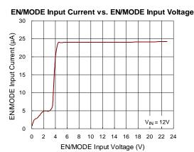
Figure 3. Characteristics of EN/MODE Input Current
