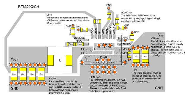
Figure 19. RT6320C/CH Layout Guide
