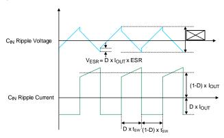
Figure 13. CIN Ripple Voltage and Ripple Current
