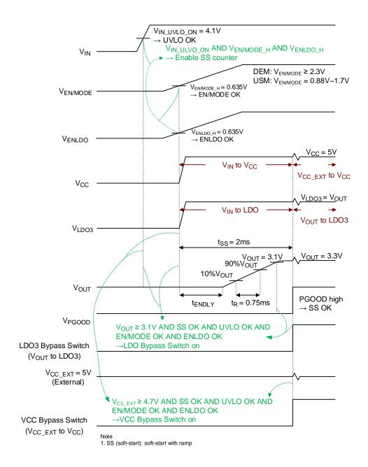
Figure 4. The RT6320B/BH VIN and EN/MODE Pin Power On
