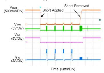
Figure 3. Short-Circuit Protection and Recovery
