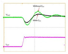
Figure 11. Load Transient Response with and without **Feedforward Capaction**
