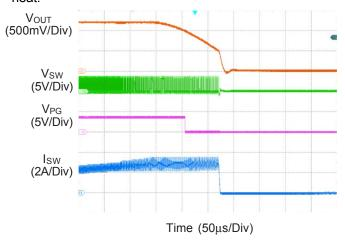
Figure 2. Over-Current Protection
