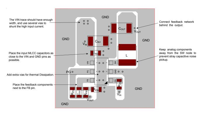
Figure 12. Layout Guide for TSOT-23-6
