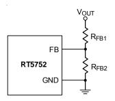
Figure 5. Output Voltage Setting
