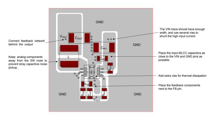
Figure 13. Layout Guide for WDFN-6L 2x2
