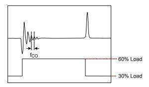
Figure 10. Example of Measuring the Converter f<sub>CO</sub> by Fast Load Transient
