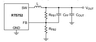
Figure 9. Feedback Loop with Feedforward Capacitor
