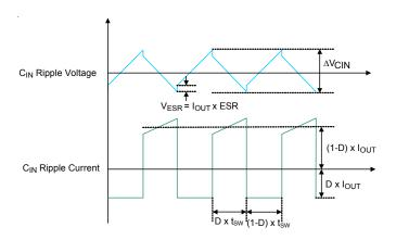
Figure 4. C<sub>IN</sub> Ripple Voltage and Ripple Current
