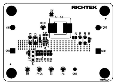
Component Placement Guide—Component Side (1st layer)
