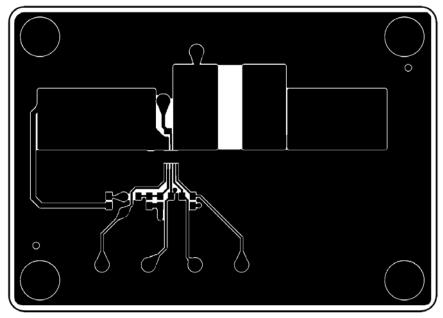
PCB Layout—Component Side (1st Layer)
