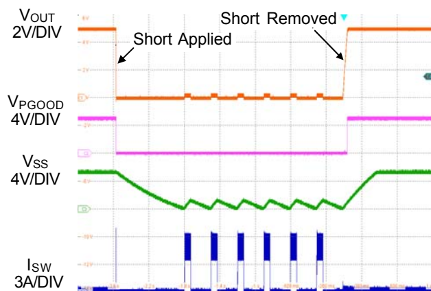
Figure 3. Short-Circuit Protection and Recovery
