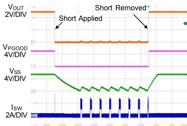
Figure 3. Short-Circuit Protection and Recovery
